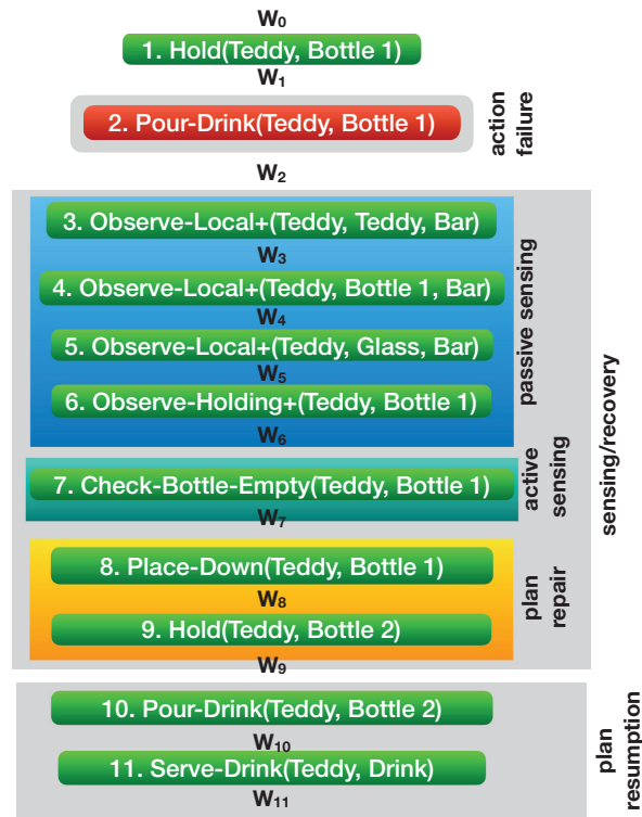
Figure 3.3. A solution plan for the Drink Refill domain's planning problem. Green actions are successfully performed actions. Red actions are ones that are attempted but that fail because their material preconditions are not all met in the world state where they are attempted.
